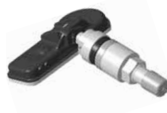
Moment mutter 8.0 Nm Moment ventilnål 0.4 Nm
