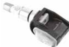
Moment mutter 8.0 Nm Moment ventilnål 0.4 Nm
